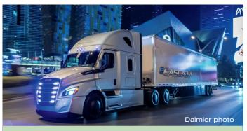
The eCascadia is an electric version of Daimler's Freightliner line, its most popular long-haul truck.
